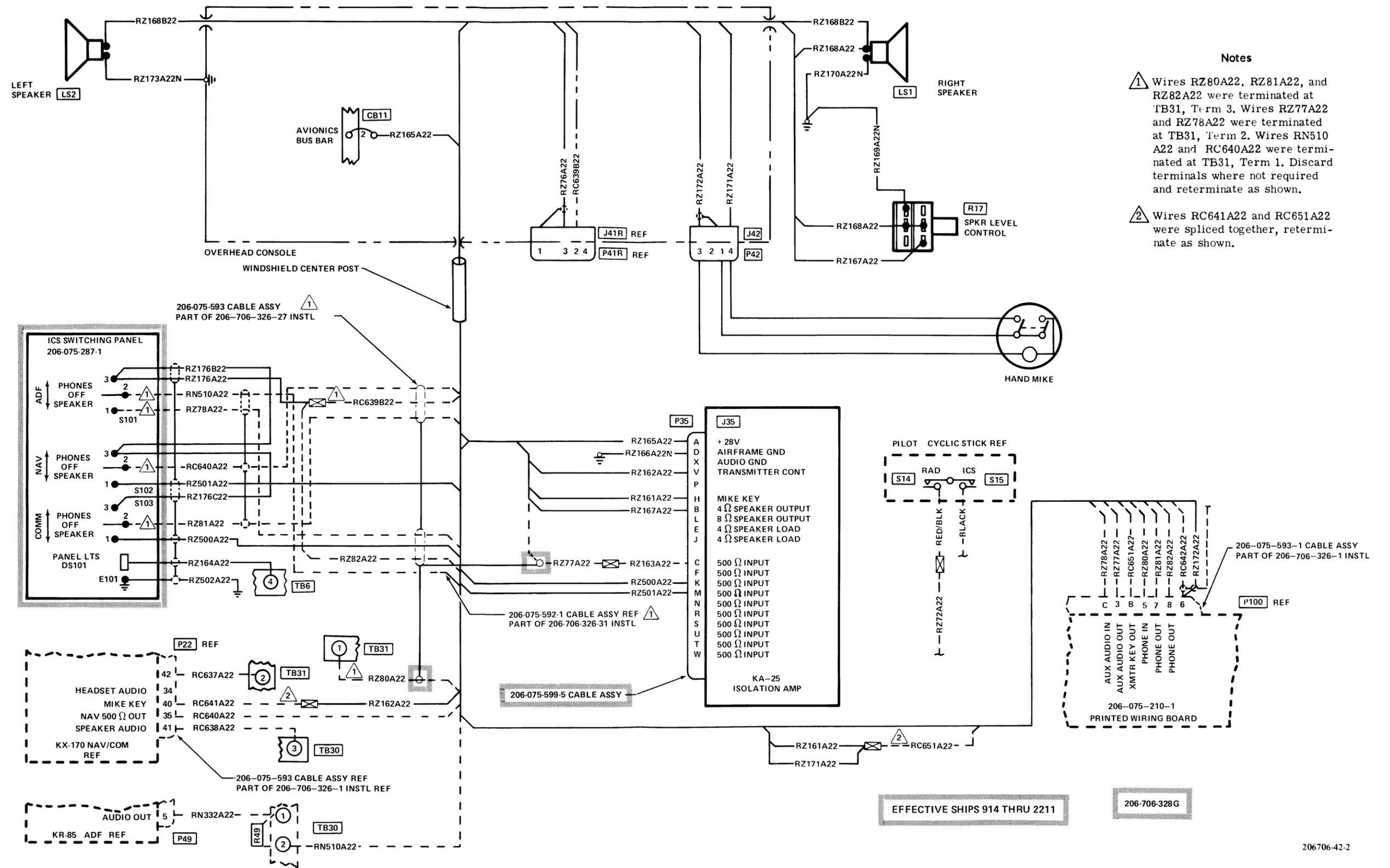
Figure 12-2. Auxiliary Equipment Wiring Diagram — Cabin Speaker (Sheet 2 of 2)
