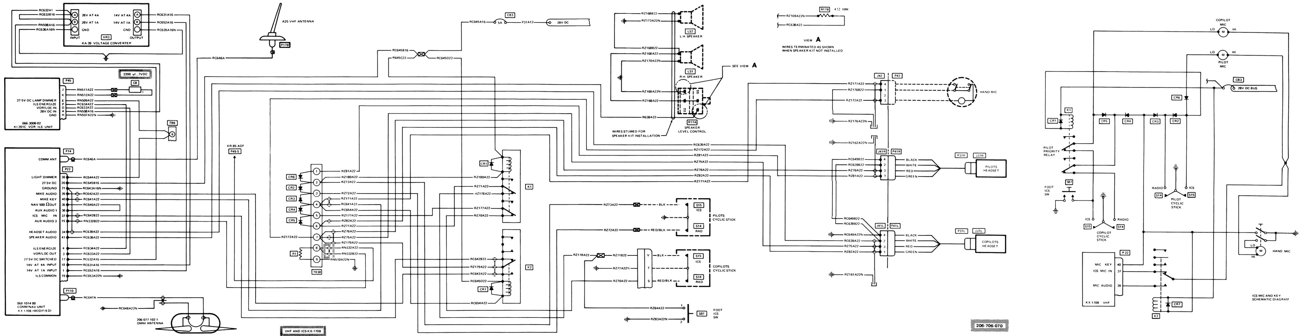
Figure 12-1. Auxiliary Equipment Wiring Diagram — VHF NAV/COMM and ICS (King KX-170B) (Helicopters 2564 thru 2166) (Sheet 4 of 4)
