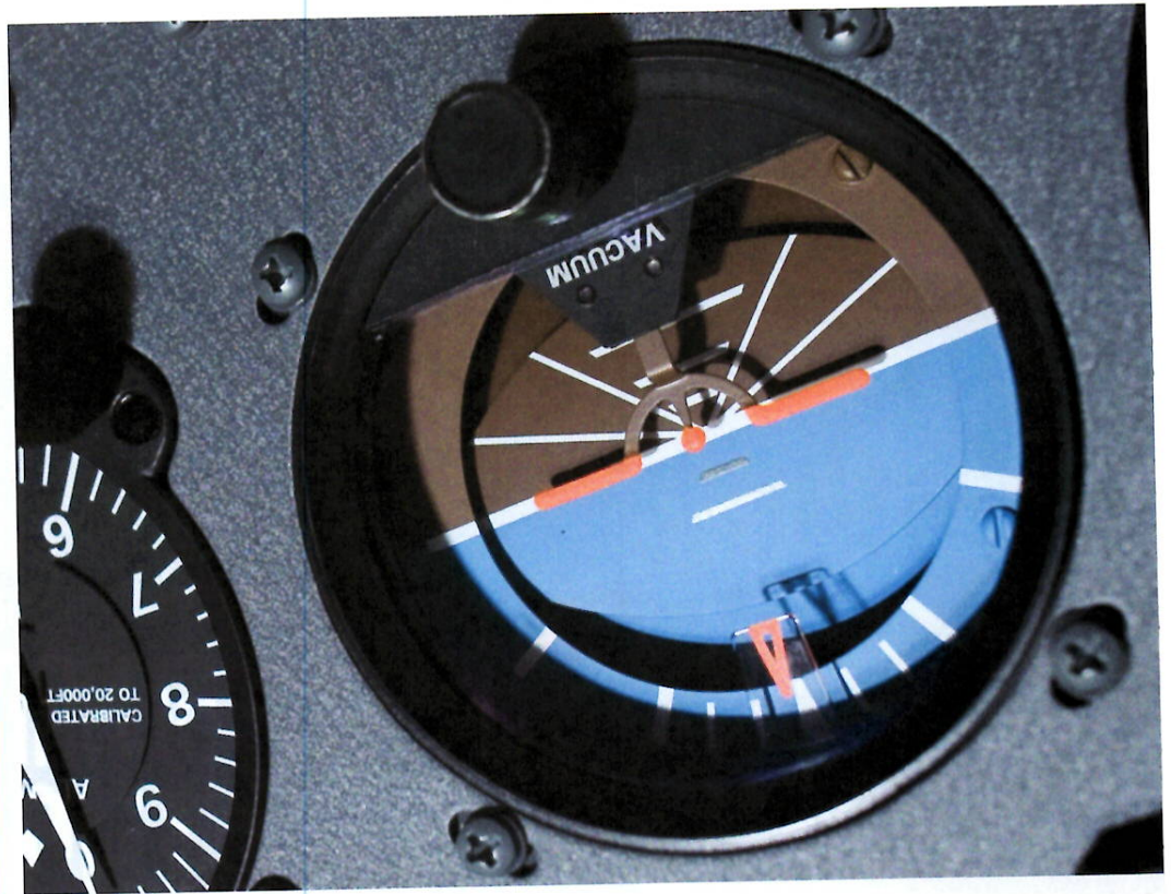
Traditional attitude indicator A blue sky, a brown ground, measurements for pitch and bank, and a mechanical gyro in the back.
