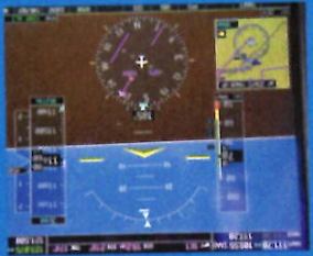
Primary flight display The primary flight display takes all the basic flight parameters, including speed, heading, yaw, attitude, and vertical speed and plasters them on a screen in which the attitude indicator takes center stage.
