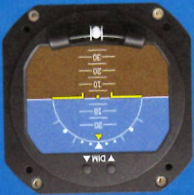
Traditional attitude indicator A blue sky, a brown ground, measurements for pitch and bank, and a mechanical gyro in the back.
