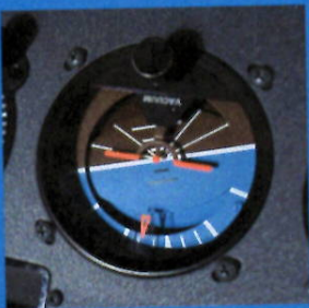
Traditional attitude indicator A blue sky, a brown ground, measurements for pitch and bank, and a mechanical gyro in the back.
