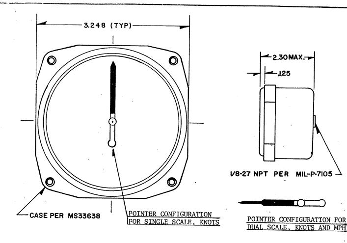
UNITED INSTRUMENTS, INC. **RANGE** PART NO. CODE NO. 8000 B.445 0 - 130 KNOTS 8000 B.463 0 - 130 KNOTS, 0 - 150 MPH 8000 B.446 0 - 170 KNOTS 8000 B.464 0 - 170 KNOTS, 0 - 200 MPH8025 B.477 0 - 200 KNOTS 8025 B.488 0 - 200 KNOTS, 0 - 230 MPH8025 B.447 0 - 210 KNOTS 8025 B.465 0 - 210 KNOTS, 0 - 250 MPH8030 B.448 0 - 260 KNOTS 8030 B.466 0 - 260 KNOTS, 0 - 300 MPH8040 B.480 0 - 350 KNOTS 8040 B.489 0 - 350 KNOTS, 0 - 400 MPH
