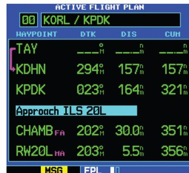
Figure 5-36 Procedure Header Highlighted
