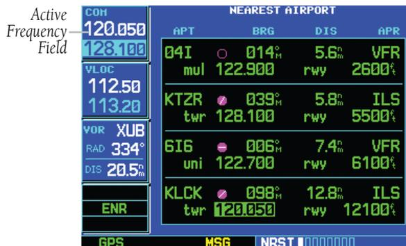
**Figure 8-8 Frequency Moved to Active Field**
