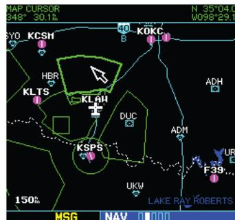
Figure 3-15 Select Airspace with Target Pointer
