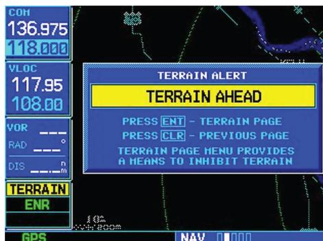
Figure 12-4 TERRAIN Caution Pop-up (Flashing)
