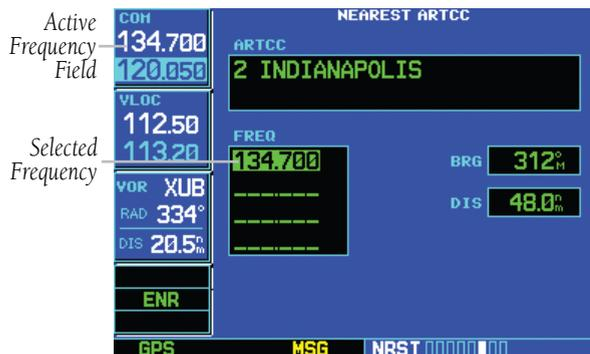
**Figure 8-18 Frequency Moved to Active Field**
