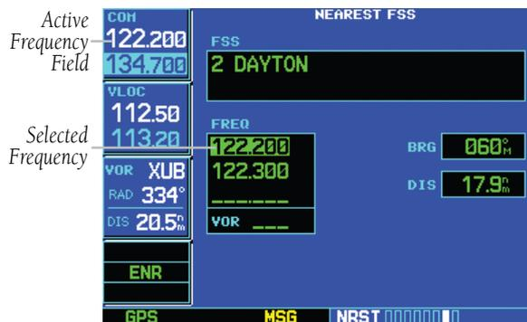
**Figure 8-21 Frequency Moved to Active Field**
