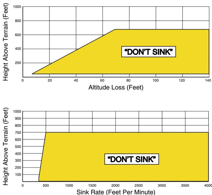
Figure 13-9 Negative Climb Rate (NCR) Alert Criteria
