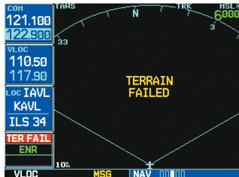
**Figure 13-11: TAWS FAILED Display**
