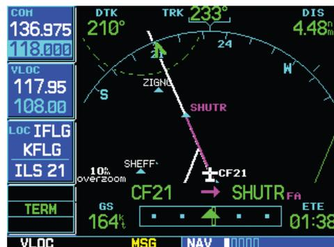
Figure 6-69 Switches to VLOC
