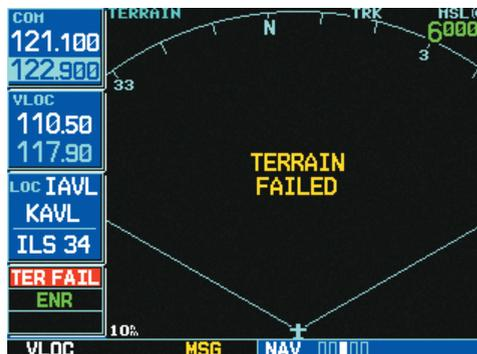
Figure 12-9: TERRAIN FAILED Display
