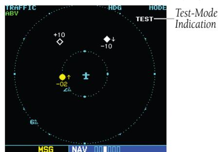
Figure 14-21 Self-Test Mode
