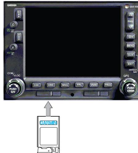
Figure A-2 Data Card Insertion/Removal Detail
