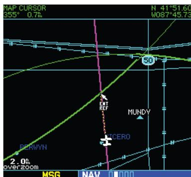
Figure 3-22 Using Pointer to Measure Distance and Bearing
