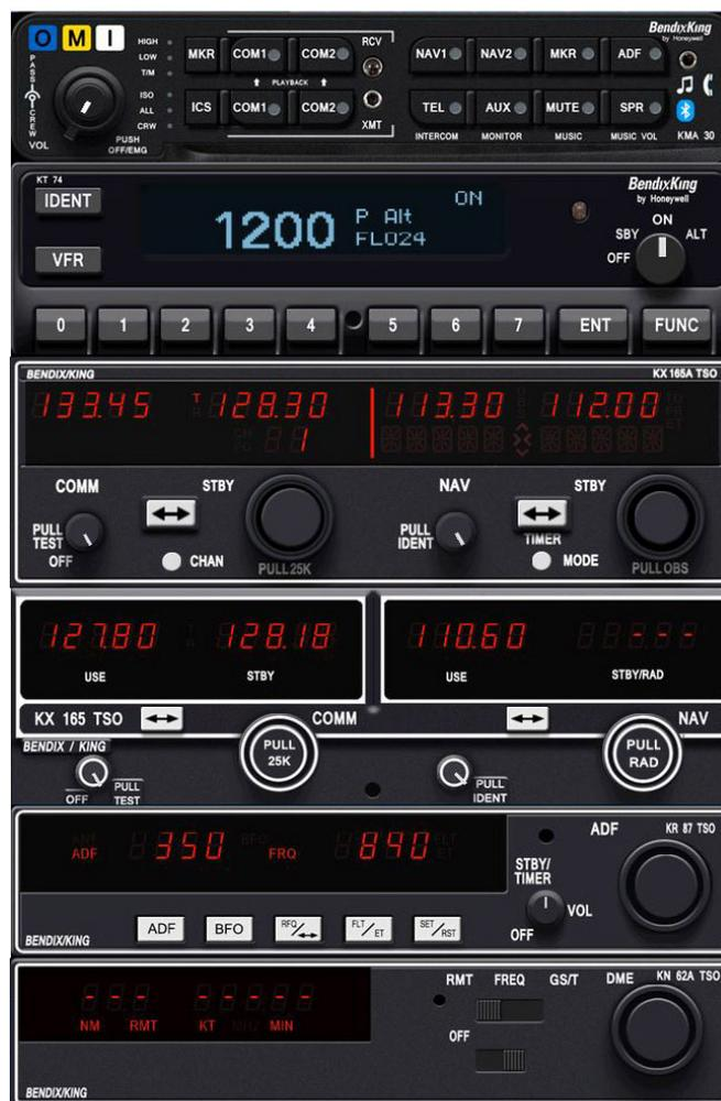
ing not only a 32 channel memory for the communication radio, but also multiple modes for the navigation radio including a CDI mode, a Bearing mode, a Radial mode, as well as a timer.
