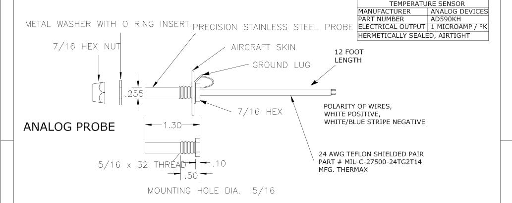
NOTES: THE TEMPERATURE SENSOR MOUNTING SHOULD BE IN A PLACE THAT IS FREE OF EXHAUST GASES OR COWL FLAPS AIRFLOW. THE IDEAL PLACE IS TWO FEET OUT FROM THE WING ROOT ON THE BOTTOM OF THE WING. SENSOR LEADS MAY BE LENGTHENED OR SHORTENED WITHOUT AFFECTING
