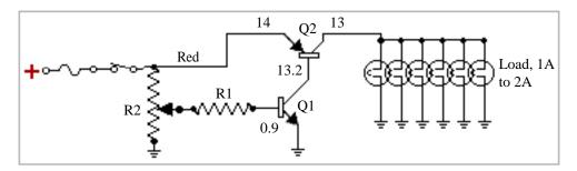
A typical dimmer circuit, capable of up to 2 amps without a heat sink, or more with a heat sink. The circuit is from RST. The voltages shown are with a 14 volt input, and R1 selected to provide 1.2 volts across the emitter and collector of Q2 when the load is 2 Amps and R2 is on full. R2 is 5k Ohms. The cost of the components, including box, is expected to be less than ten dollars. Compare that to the \$35 for a rheostat or the \$81 from Cessna for its rheostat.
