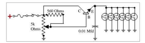
This circuit appeared as a hint for homebuilders. The 2N3055 transistor at Radio Shack is a bit over two dollars and is the most expensive part shown, though the metal box would be more. If you heat sink the transistor, using the insulator and heatsink grease, this circuit can handle up to 15 Amps, but without the heat sink it would have a limit of 5 Amps. The capacitor is to prevent amplification of bus transients which would make the lamps flicker.
