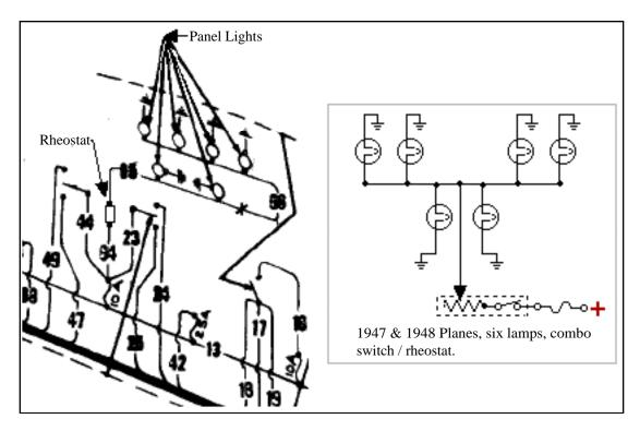
On the left, as Cessna shows the Rheostat and on the right the way the circuit should have been indicated with the switch a feature of the rheostat.
