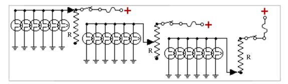
In the three circuits shown you have the three positions; A) full voltage across the lamps with the rheostat doing nothing and the lights at full bright; B) partial voltage for an intermediate intensity; and C) with the rheostat's entire resistance in the circuit and the lights as dim they can be, dependent on the ratio of the lamp resistance and the rheostat resistance.
