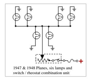
The lamps for these newer planes was the G.E. 1826; the mystery is why they chose to use an 18 volt lamp with poor life for a 12 volt system. The 1826 did use a lot less current, less than half of the previously used 1816. If they had used the same lamp as on the '46 planes, the '47 and subs would have meant they would need a larger wattage rheostat but they kept the same rheostat on all the planes and reduced the current by more than half by changing to the 1826.
