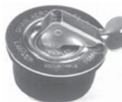
Pressure fuel caps are recommended for aerobatic installations. These caps are made with Buna-Nitrile gaskets for fuel resistance. These caps are non-vented for gravity fuel systems. It is highly recommended that a #40 (3/32") drill is used to drill a vent hole through the lower base plate and stud assembly using a drill press.
