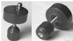
The ACS bearing regreasers restore bearings, rod ends and pulleys to "like-new" condition. O-ring in base of regreaser provides positive seal when bearing is secured by the threaded center post. Grease, entering under pressure at the grease fitting, is forced to flow through the bearing, flushing out the old grease and dirt, and recharging the bearing with fresh grease. Anodized aluminum construction. Available in five sizes.
