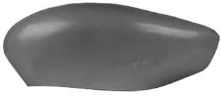
**MF-1A** - 5:00 X 5 fairing that is small and compact. The same shape and size as the early model Cessna 150 & measures 26" long by 7" wide. Has been used on the CA-61, Tailwind, T-18, Baby Ace, Cougar, or any home-built that requires this size.
