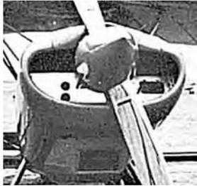
Styled after the Piper Comanche, this cowl can be used on just about any homebuilt powered by the Lycoming engine. It is made in two parts, allowing the easy removal of the cowl without having to remove the prop. Used on the following airplanes: Starduster I and II, Playboy, EAA BiPe, Jodel D-11, Tailwind, Tempete & the Skybolt. Measures 35" wide by 21" high. Will accommodate a spinner approx. 12" in dia. P/N MC-1A .....\$72.50
