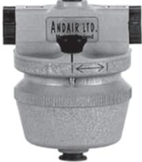
Andair has developed this tough and compact gascolator with some great features. They are suitable for engines up to 140 HP and act as a trap to catch water. A unique method of attaching the bowl to the body allows for real easy maintenance. By pulling out the locking safety pin then rotating the bowl through 35°, bowl can be pulled off and the internals inspected. It literally takes 30 seconds!
