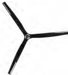
The In-Flight Adjustable Pitch Ivoprop allows the pilot to change the propeller pitch in flight through a toggle switch mounted in the cockpit. Pressing the toggle switch one way sends an electric current through the graphite brushes to the slip rings and finally to an electric motor. Torque from the electric motor is channeled to a planetary gear drive which turns the lead screw. Torsional rods transmit movement from the center
