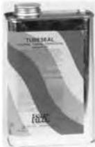
Prevents rust and corrosion inside aircraft tubing structures. Tubeseal is a blend containing a very fine preservative oil (MIL-L-21260) which has a characteristic of climbing the tube wall and spreading over the entire surface to provide lasting protection. Penetrates and reveals very small pin holes in a weld and in time, due to exposure, congeal and seal the hole. 1 quart will treat 2 light aircraft fuselages. Complete instructions on label.
