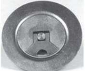
The UD-3 flush fuel cap assembly is an unvented cap similar in design to the #5 style cap. The aluminum mounting ring has a 2" dia. opening and an overall dia. of 3-3/4". It may be riveted, bolted or molded to the tank. It is currently used on many popular homebuilts such as the RV's, Lancair, Velocity & White Lightning. Specify flat or contoured adapter.
