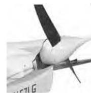
This super-light spinner dome weighs about 8oz. which drastically reduces the spinner assembly weight and the need for lead ballast in the nose of pusher-type aircraft. This weight savings, combined with the revolutionary new tapered spinner dome which reduces drag can increase the cruise speed of almost any pusher-type homebuilt. These spinners have been used on a modified VariEze to win several air races.
