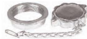
Locking bayonet type cap with gasket, fastens to filler neck with safety chain. Externally threaded to mate with tank flange. 1.5" dia. filler hole, 2.25" diameter at threaded base, 1-3/8" neck length. Complete with aluminum tank
