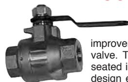
This J-3 fuel valve includes a steel handle for use with the original pushpull shut off control. this valve is a significant improvement over the original brass style fuel valve. The new valve has a stainless steel ball seated in an inert composite seat. This improved design eliminates the stiff operation and leaking around the shaft that the original design was prone to. PMA approved.
