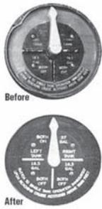
This fuel selector plate is billet machined and anodized, with the text engraved on the plate. It is an efficient one piece design which is easy to install and factory guaranteed. FAA/PMA approved.
