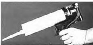
These air-powered dispensing guns are recommended for applying Pro-Seal type sealants in larger quantities and where positive control of the material being dispensed is critical. The unit's rugged construction makes it ideal for in-plant production applications that may require full line air pressure. Features include twist lock instant loading, smooth dispensing, non-bleeder application control and positive application control. Lightweight.
