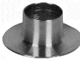
Simplify installation of cabin, carb. heat, cabin vent lines. Aluminum flange may be welded or riveted in place. Slip ducting over outlet and secure with clamp.
