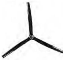
The Quick Adjust System Ivoprops allow you to adjust the pitch on the ground in a matter of seconds by turning the screw adjuster in the center of the prop. The supercams are installed on the square end of the torsional rod. Each supercam fits into the groove in the screw adjustor. Turning the screw adjustor causes each cam to rotate and turn the torsional rod and
