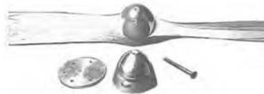
For all props with standard Rotax® 75mm bolt pattern. Spinner bulk head is predrilled and installs between prop and gearbox flange. Spinner installs with single bolt.
