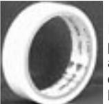
ISD Chafe Tape is a durable Teflon material with a pressure sensitive adhesive which resists solvents, and oils. Designed specifically to prevent aluminum chafing between airframes and engine cowls. It helps prevent black streaking on aircraft exterior due to cowl chafing and is FAA/PMA approved. Operable temperature range: -100°F to +500°F. Width: 1". Roll length: 6 yds. Tkns: .012"
