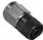
Aeroquip 471 hose fittings consist of an AN818 nut, an externally threaded 37° nipple and an internally threaded hose socket. All components are anodized aluminum. Fittings conform to MS27404.
