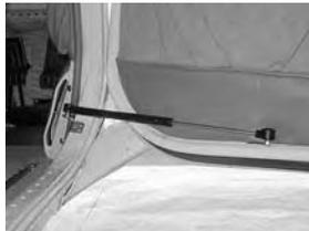
The **DOOR STEWARD™** is an STC & FAA-PMA approved modification that greatly improves and replaces easily broken, malfunctioning mechanical type door stop or restraints that become ineffectual with repeated usage.
