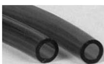
This fuel line is blue in color and does not rot or deteriorate from the inside, clogging the carburetor or fuel system. It withstands 50 PSI and tensile strength is 8000 PSI. It is resistant to temperatures of -65° to 220°F without deterioration, features exceptional resistance to gasoline, oil, oxygen, and ozone, and has high elastic memory allowing use of Delrin or nylon barbed fittings in low pressure applications without the need for external clamps.
