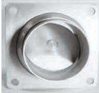
Made from 6061 aluminum and anodized these vents are made to give long trouble free service. The mounting flange is 2.2" square with a mounting hole pattern of 1.70". The air flows through a 1.2" hole allowing this vent flow more than most "small vents."
