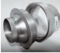
Made from 6061 aluminum and anodized these vents are made to give long trouble free service. The mounting flange is 2.25" round with a mounting hole of 2.0". The vent comes with a hose adapter that screws to the back of the vent, securing it in place. This hose adapter allows you to connect a 2 inch hose directly to it. The air flows through a 1.2" hole allowing this vent flow more than most "small vents."
