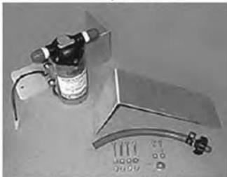
Smoking airplanes smoke system bracket for mounting the oil pump on the side OR end of the SA-102 and SA-103 Oil Tank. The oil pump bracket is perfect for areas where the top mounted oil pump is too tall to fit your needs. The bracket is 1/8" thick aluminum with all holes pre-drilled. All hardware is provided for a complete conversion including a pre-fitted suction hose extension with fittings.
