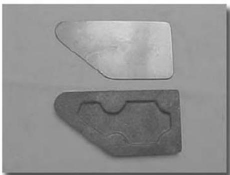
Spar to Fuselage Attach Fitting (Casting)
