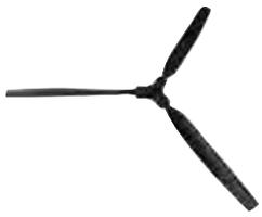
**Warp Drive's Advanced Composite Carbon Fiber propeller has a structural strength near that of metal propellers.** Because of the stiffness achieved by using carbon fibers, the prop will do very little coning (bending forward) under power. Proper fiber placement allows the prop to flex torsionally for maximum cruise efficiency.
