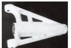
These PMA approved replacements for the Nose Gear Brace are used in early Bonanzas. Most of these aircraft have severely corroded nose gear braces as a result of lightening holes that allow moisture to enter and collect in the bottom of the housing. Even dry country aircraft are found to have corrosion. This is because many of these aircraft have been repainted and paint remover has entered the housing and is reactivated when water enters the housing during aircraft washing.
