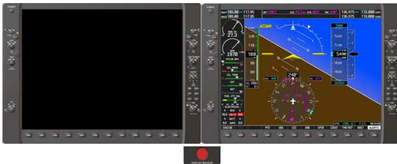
Figure 14.5 – Using the reversionary button to recover a failed PFD
