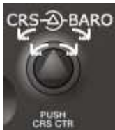
Figure 5.10–CRS and BARO Selection knob
