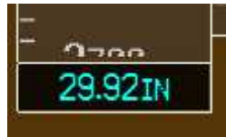
Figure 3.12 – Altimeter setting read under Altimeter vertical tape
