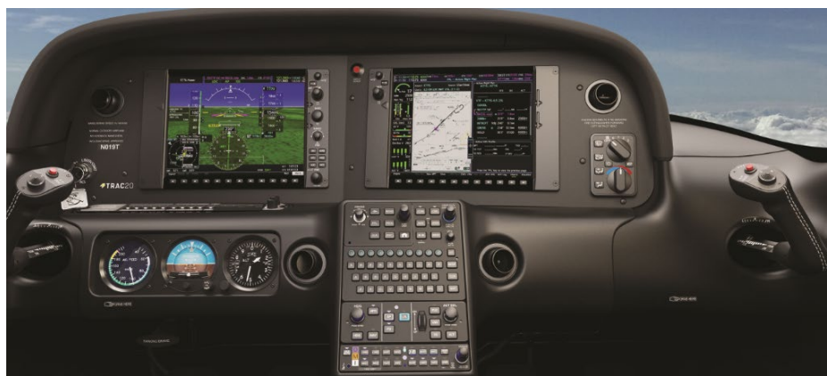
Figure 3.1 – Cirrus Sr-20 Garmin Perspective cockpit layout
