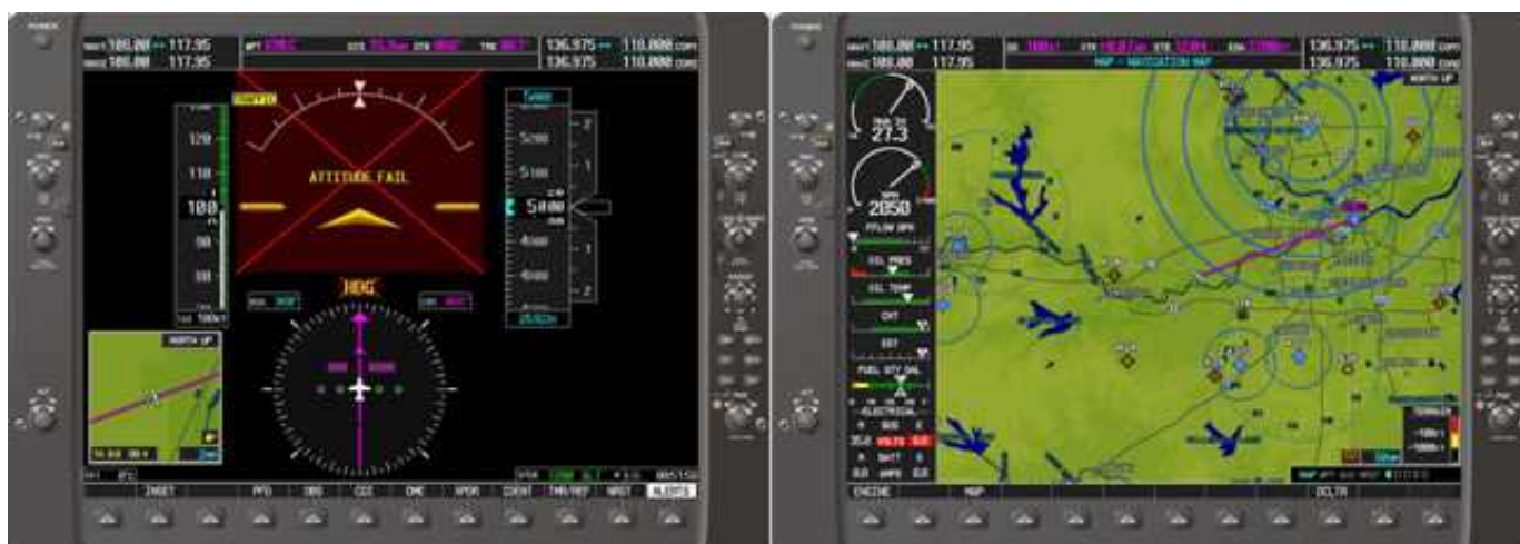
Figure 14.2 – GRS77 AHRS failure
