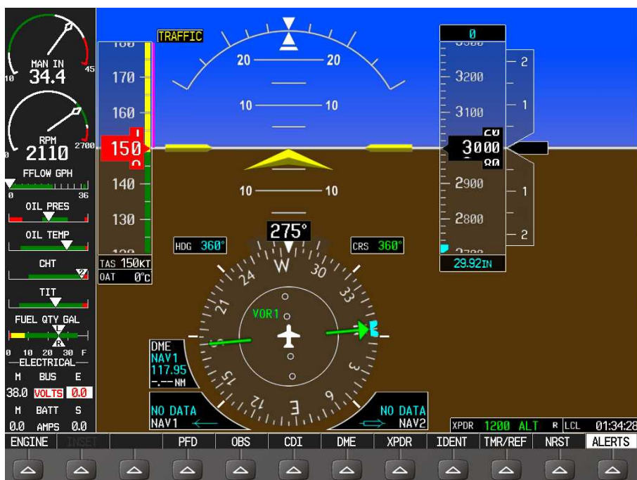
Figure 8.9 – The G1000 in reversionary mode
