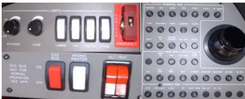
Figure 14.7 – The power distribution bus and backup battery switch on a Diamond DA40 aircraft
