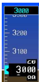
Figure 3.10 – ALT bug has no bump function and must be twisted
