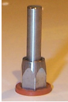
Figure 2.14 – The GTP 59 OAT Probe sensor
