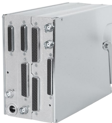
Figure 2.7 – The GIA 63 Integrated Avionics control box
