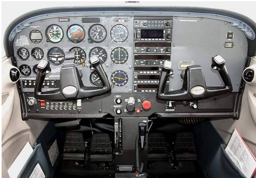
Figure 1.3 – Traditional aircraft panel (2002 Cessna Skyhawk SP)
