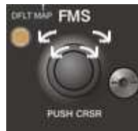
Figure 13.4 – Use FMS knobs to select option
