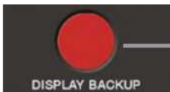
Figure 8.8– The GMA1347 Reversionary mode button
