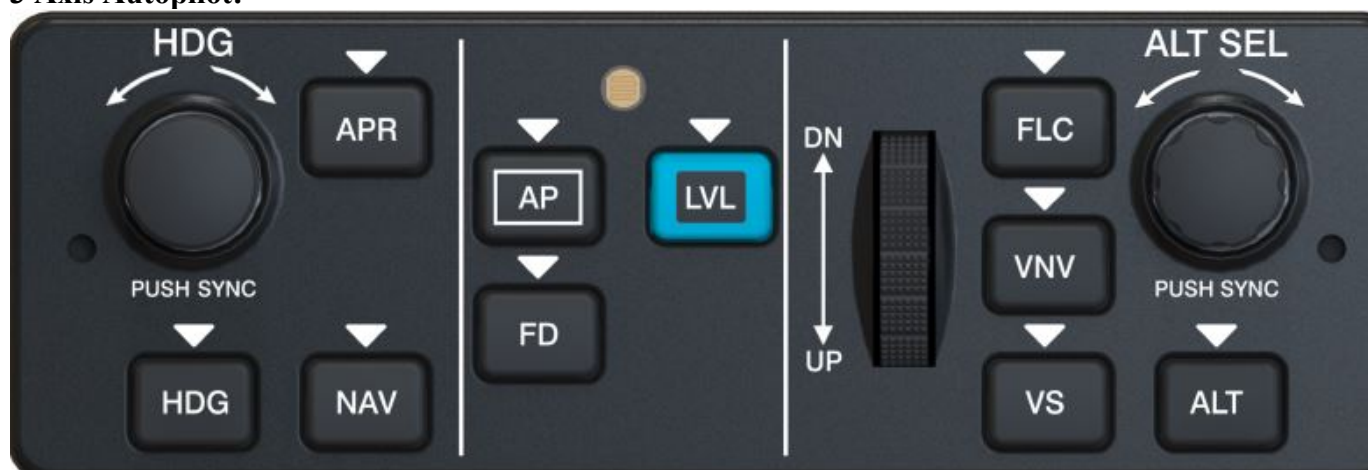
Figure 12.2 Integrated Garmin Perspective Plus Autopilot Control Panel
