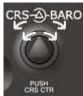
Figure 5.27–CRS knob used to set OBS course heading
