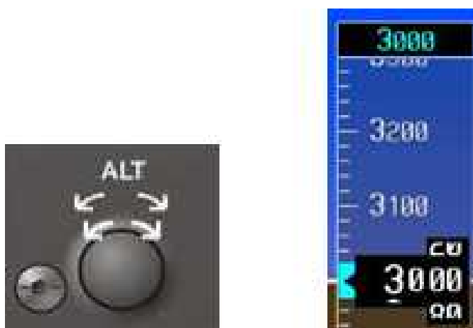
Figure 12.9 Using the ALT knob to set a reference altitude of 3000 feet
