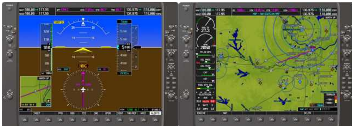
Figure 14.4 – GMU 44 Magnetometer failure
