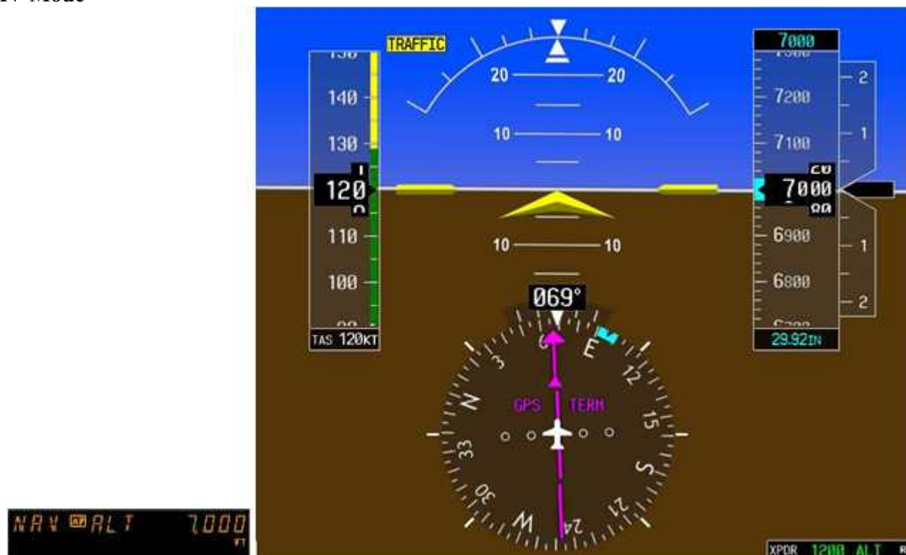
Figure 12.10 Autopilot in NAV mode tracking GPS needle in GPS
