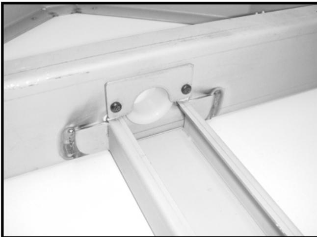
**6.** Mount the nylon bearing in the middle of the frame and secure it with the small bracket. You will need a Torx H10 screwdriver for the self tapping screws.
