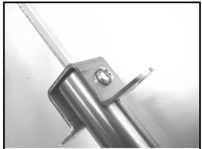
**28.** Now mount the slider bracket onto the yoke tube using 2 M4 bolts.
