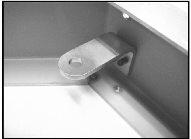
**20.** Now mount the larger bracket onto the right inner side of the yoke frame. Leave the upper holes free. They will not be used.
