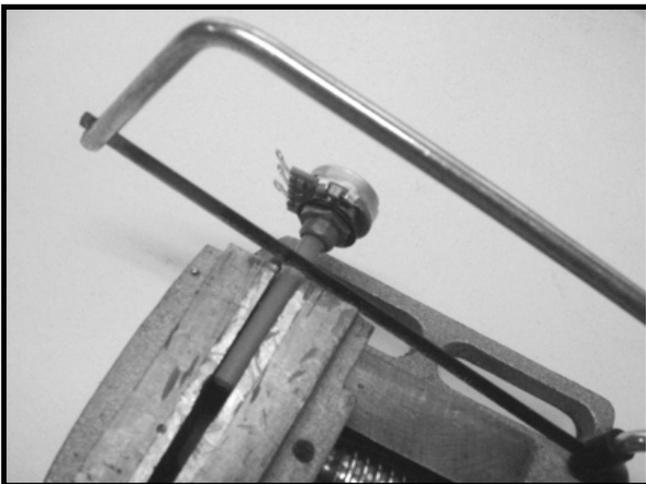
**1.** The potentiometer for the Roll movement has to be shortened to 12 mm. Cut it with a small saw to length.
