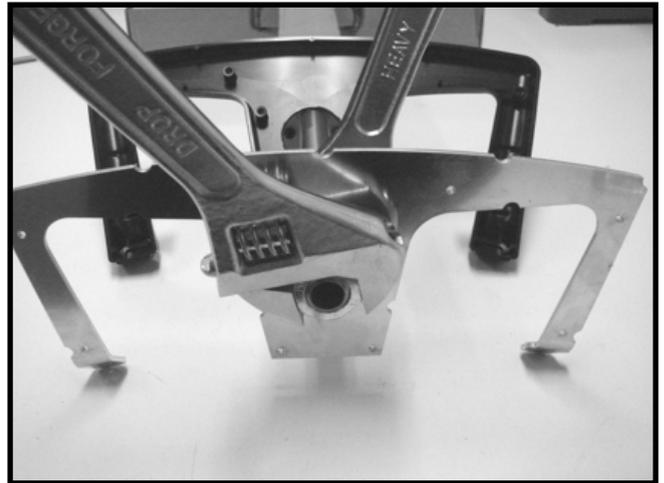
**44.** Now tighten both nuts on the yoke tube firmly, but be sure that the position of the tube and the frame does not change!
