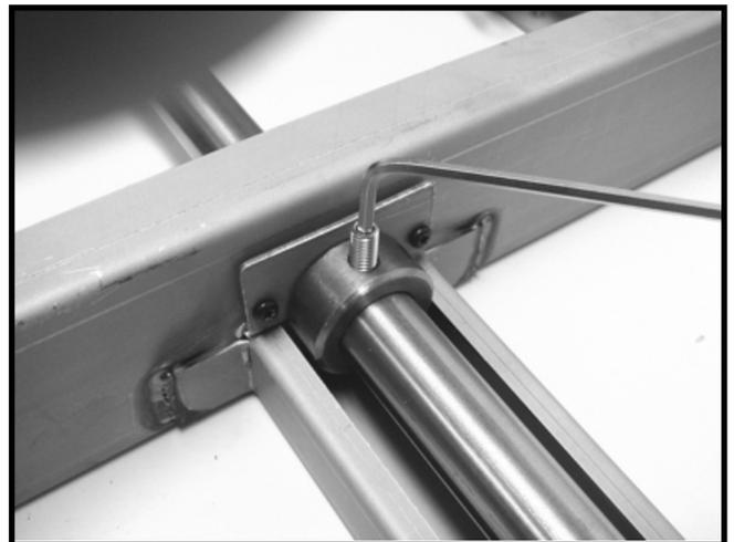
**34.** Tighten the yoke tube ring using the inbus bolt. **VERY IMPORTANT: the yoke tube and the yoke bracket must be hold in the positions as indicated in picture 32 and 33.**
