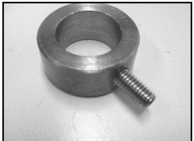
**22.** Mount the larger inbus bolt just enough not to loose it, but leave the inside of the ring open to let the yoke tube pass.
