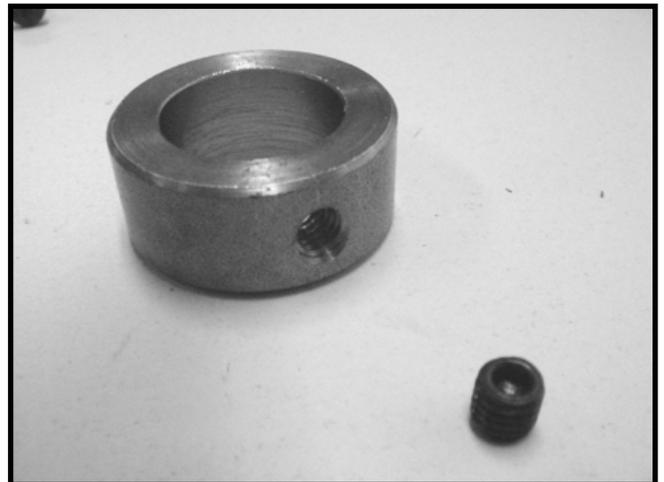
**21.** Unscrew the inbus bolt from the yoke ring (when supplied). The smaller inbus bolt is of no use anymore.
