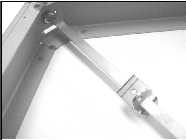
**24.** Position the yoke slider over the flattened end of the potentiometer shaft and mount by hand the small black screw just enough that the screw holds.
